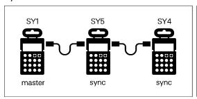
example A: sync three pocket operator units. chain: PO-12 > PO-24 > PO-33
