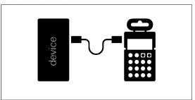
if a cable is inserted into the line in jack, the PO-33 will record via line in.
