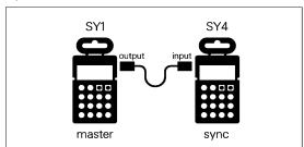
it is possible to sync multiple pocket operators with a click track using line in and out.
