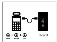
sound and pattern data can be stored to any stereo recording device for saving and sharing. connect a 3.5mm stereo cable from the transferring unit line out to the recording device line in.
