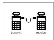
it is possible to transfer sound and pattern data directly between units, using the line out / line in connectors.
