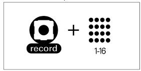
hold record + any key from 1-16. the microphone will record until the keys are released, and the recording will be stored in the position you selected (1-16). PO-33 has a total of 40 seconds recording memory, while recording, the number of seconds left will be displayed on the LCD. if the memory is full, delete or record over an existing
