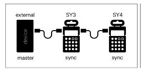
example C: sync an external device to two pocket operator units.
