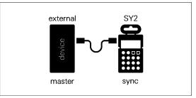
example B: sync external device such as volca, iPhone, computer or synckontrol to PO-33.
