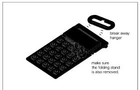
to mount the pro case to a pocket operator, first you need to break away the hanger and remove the folding stand.
